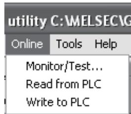
[Monitor/Test]: Activates the Select monitor/test module screen.
